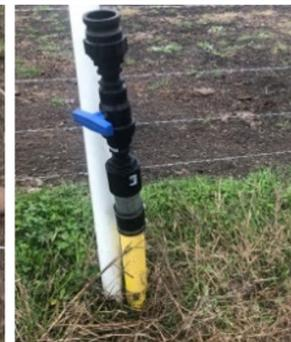
The issue now was that the hose clamps on the boot weren't strong enough. Because of the back pressure, we probably shot that vent/hose attachment off the vent about 5-7 times. In the end two additional hose clamps were added to hold the hose attachment to the casing. The entire volume of slurry in the tank was pumped, but only three pails of PGH-400 gel was added through the hopper. The installation was successfully completed.
