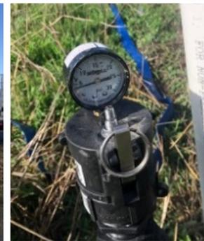
Because of the large amount of water in the casing, backpressure was generated during the injection. There was not enough pressure from the pump to be able to use the hopper. Four pails of PGH-300 gel had been added to the tank, and an additional 1.5 pails of PGH-400 was also added since it could not be added through the hopper. An additional 200 gallons of water was added to the tank to allow for the additional gel to be pumpable.
