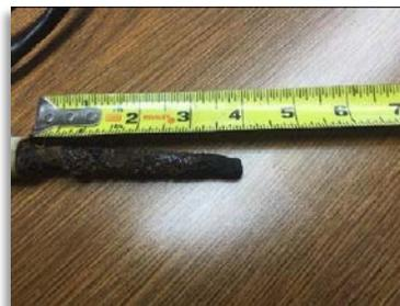
*Corroded ER Probe*
