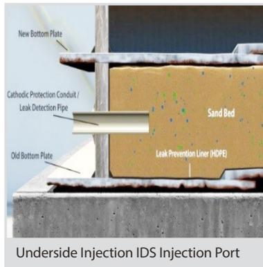
Underside Injection IDS Injection Port
